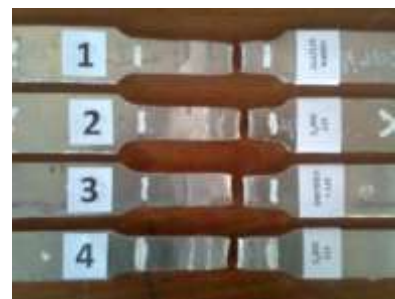
Gambar 11. Hasil uji tarik : (1) tanpa perlakuan, (2) preheat 200°C, (3) STT 200°C, (4) TTT 200°C.
