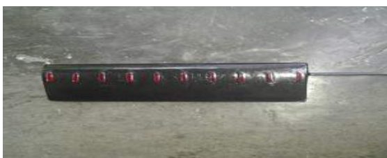
Gambar 3. Model airfoil tanpa vortex generator
